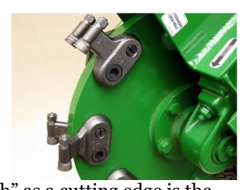
A tough carbide concave "dish" as a cutting edge is the innovative design that allows Greenteeth® to actually "sheer" rather than "shred". The sheering is a smoother motion that requires less power exertion from the machine and allows faster, more efficient stump cutting.
